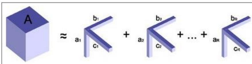
Fig. 1 In the canonical product format an n-dimensional tensor is represented as a Kronecker product of m vectors, m being the decomposition rank of the tensor.
