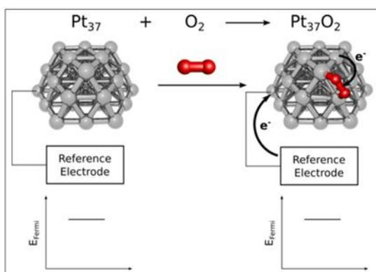
Fig. 3 In contrast to a constant charge approach, the constant potential approach is based on a SCF scheme with a fixed electrochemical potential and a variable electron number.
