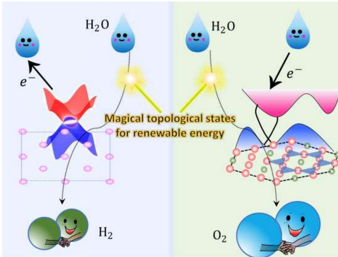
*Topological non-trivial surface states can accept or donate electrons during the water electrolysis process.*
