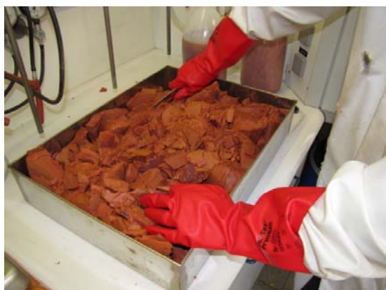
Fig. 3. Pilot-scale production of micro/meso-porous carbon aerogel. Here the production of the resorcinol-formaldehyde precursor gel is shown.
