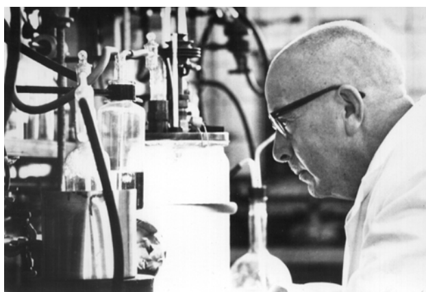
The “Ziegler-Polymerization” on a laboratory scale. The snow-white powder filling the conserving jar is polyethylene.
